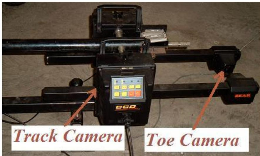
Track cameras take a reading along the side of the vehicle. Toe cameras take a reading across the front on six sensor machines. On eight sensor machines toe cameras take a reading across the front and rear of the vehicle.
